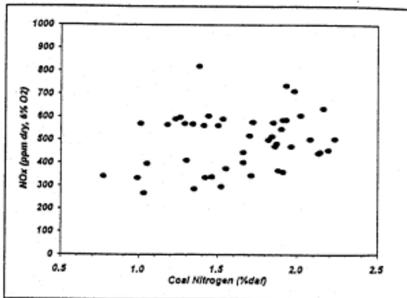
**Figure 4 Relationship between NO<sub>x</sub> Emissions and Coal Nitrogen Content (ACIRL Limited)**
