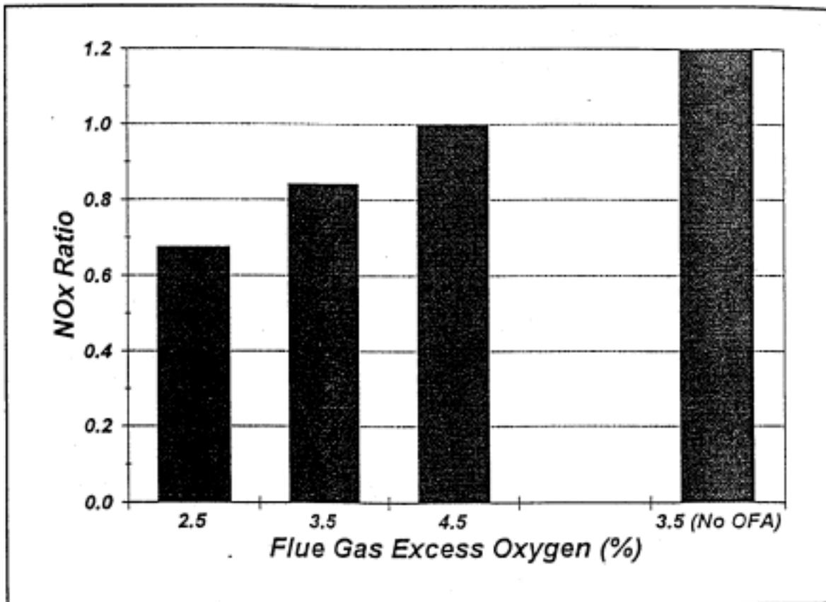
**Figure 2 Effect of Excess Oxygen and Over-Fire Air on NO<sub>x</sub> Emissions at Bayswater Power Station**
