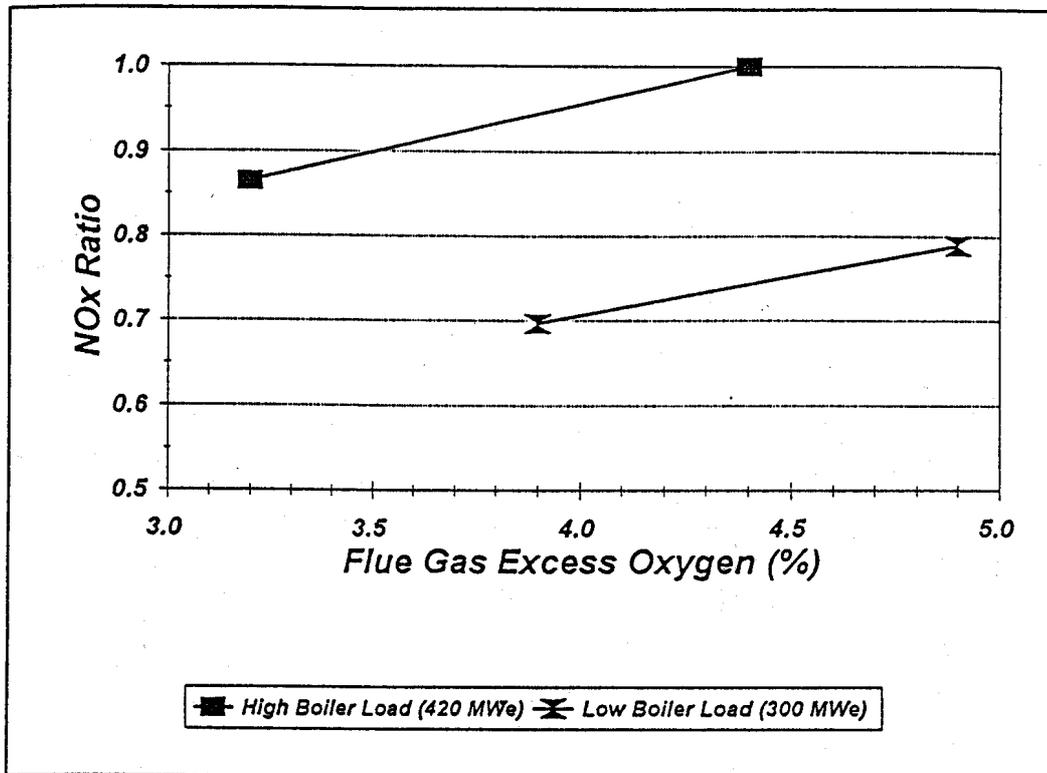
**Figure 1 Effect of Excess Oxygen on NOx Emissions at Liddell Power Station**
